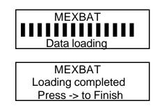
Repeat the data loading procedure if you wish to load data to the next device of the same model, and press "->" key in order to finish or to select another model of target device.
